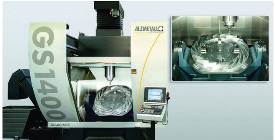
Turning and milling on 5-axis machining centre GS 1400/5-FDT – Productivity through hybrid machining in one setting (source: ALZMETALL)
