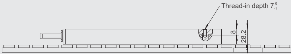
Dimensions of secondary part, variant 2 Through-bore for screw M5
